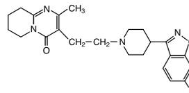
Risperidone is a white to slightly beige powder. It is practically insoluble in water, freely soluble in methylene chloride, and soluble in methanol and 0.1 N HCl.
